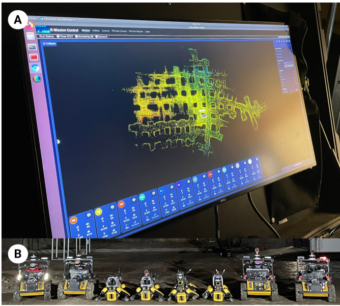
Figure 1: Team CoSTAR’s Mission Control user interface (A). (B) a subset of CoSTAR’s ground robots showing four customized Boston Dynamic’s Spot and Clearpath Husky powered by JPL’s autonomy platform NeBULA. Typically a deployment of 4 to 6 ground vehicles was targeted during SubT, but the number of agents is extendable (e.g., see A with 11 robots).
