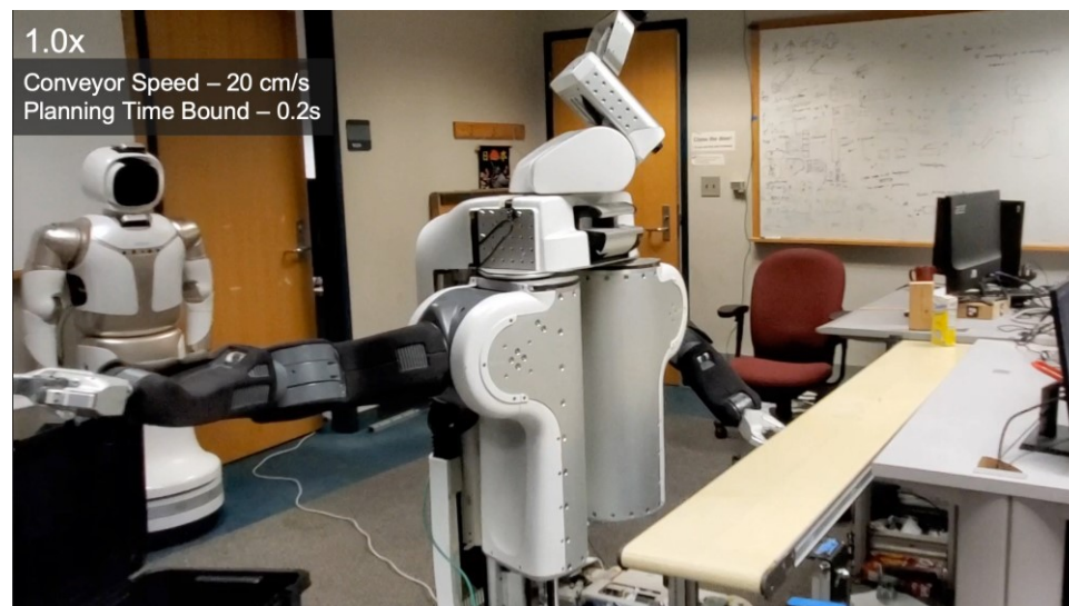
CTMP for picking dynamic objects off a conveyor with imperfect perception [Islam et al., RSS'20]
